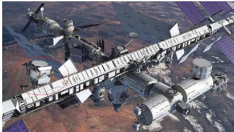
Figure 4.1: AMS-02 on the upper Payload Attach Point on S3 Truss of the International Space Station[98].
