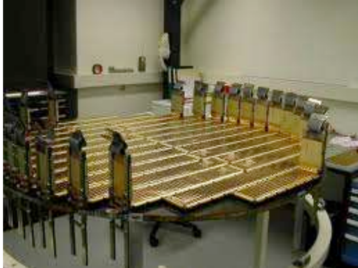
Figure 4.14: One of the nine layers that constitute the AMS Tracker system[98].
