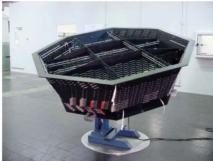
Figure 4.3: View of the TRD integrated before its installation on the whole detector[188].
