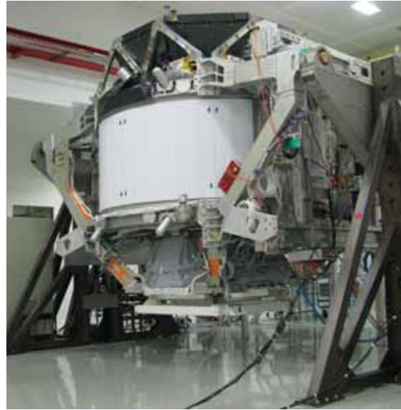
Figure 2: The Alpha Magnetic Spectrometer shuttle payload during the integration phase inside the clean room at CERN.
