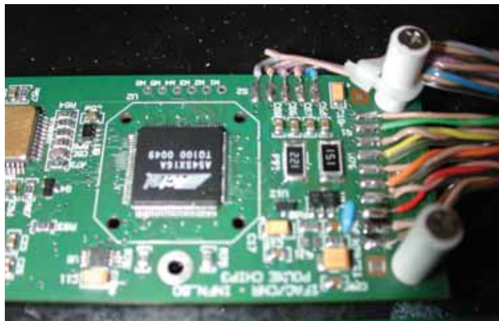
Figure 3.15: The SFEC board is powered by the five connections on the top of the figure: ground, -5V, +3.3, ground and +5V. We can see on the right all the LVDS links, that are: two for the input clock, two for the data of the first chip and two for the strobe, two for the data of the second chip and two for the strobe.
