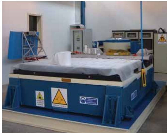
Figure 5.23: The vibration test of the lower TOF will be done with the SERMS vibration chamber shown in this figure.
