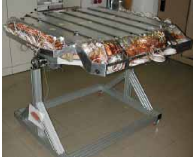
Figure 5.18: The assembly of the lower TOF detector has already been started in the Bologna INFN laboratories.
