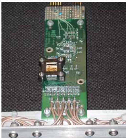
Figure 4.3: The third of the CMB and the first prototype of the SFEC, has a socket for the AICPPP chip in order to test and characterize all chips.
