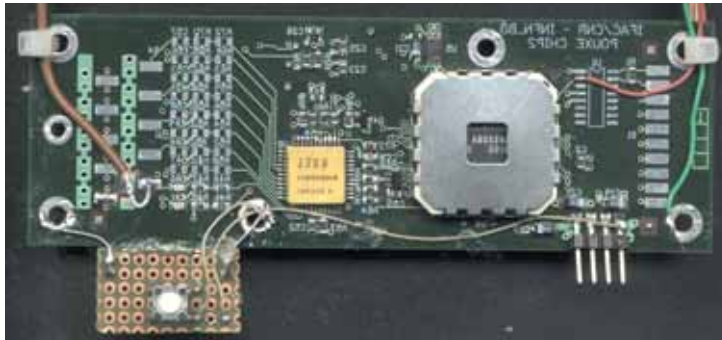
Figure 4.2: The second prototype of the CMB is composed of two AICPPP chips; one for anodes and one for dynodes, two ADCs and a socket with FPGA. The visible button on the board was used to manually reset the FPGA.
