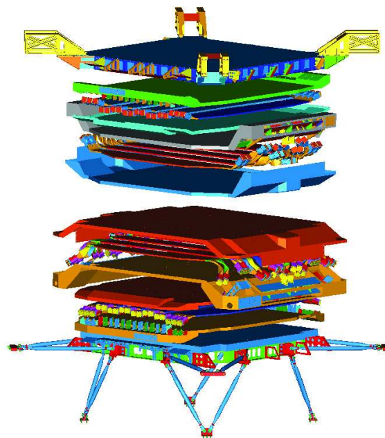
Fig. 1. Exploded view of the AMS-02 TOF subdetector.
