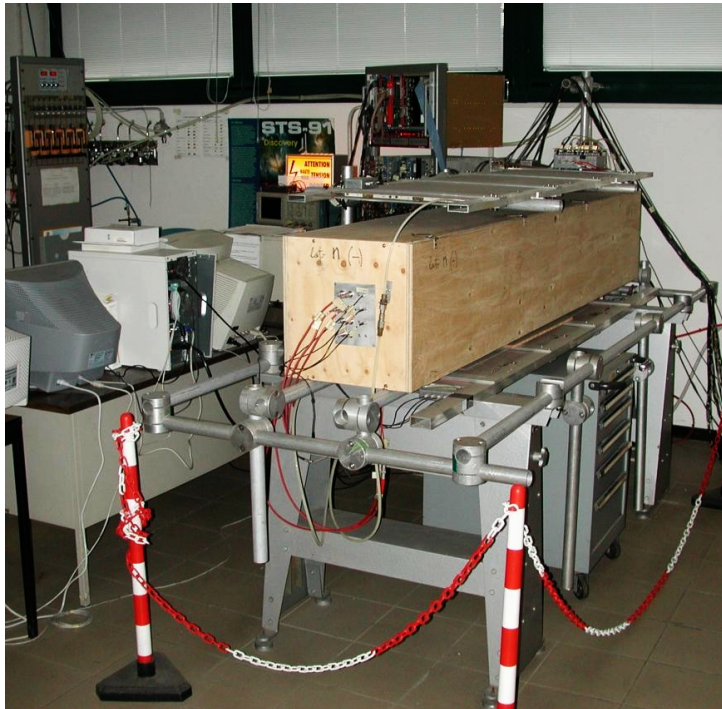
Figure 2.1: The cosmic ray telescope used for the AMS counters characterization. In the picture are shown the black wooden box, the two layers of LST above and below the box, electronics and computers for DAQ and analysis. The reference scintillation counter is under the lower LST layer.
