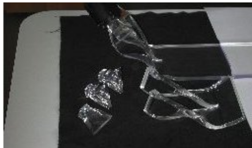
Figure 3.3: Light guides used for the TOF counters. They are tilted for the counters of plane 3 in order to minimize the influence of the magnetic field on the PMT response.
