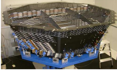
Figure 1.7: The Transition Radiation Detector (left) and the proton rejection factor during the CERN beam test (right).
