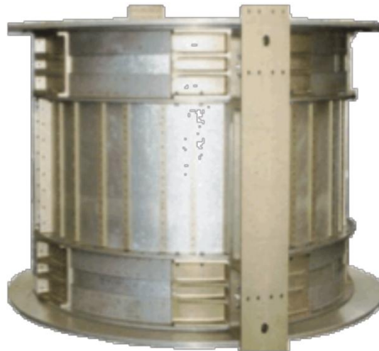
Figure 13 - The AMS-02 permanent magnet that operated [352] on board of the Space Shuttle Discovery in 1998 (Mission STS-91 - Experiment AMS-01).
