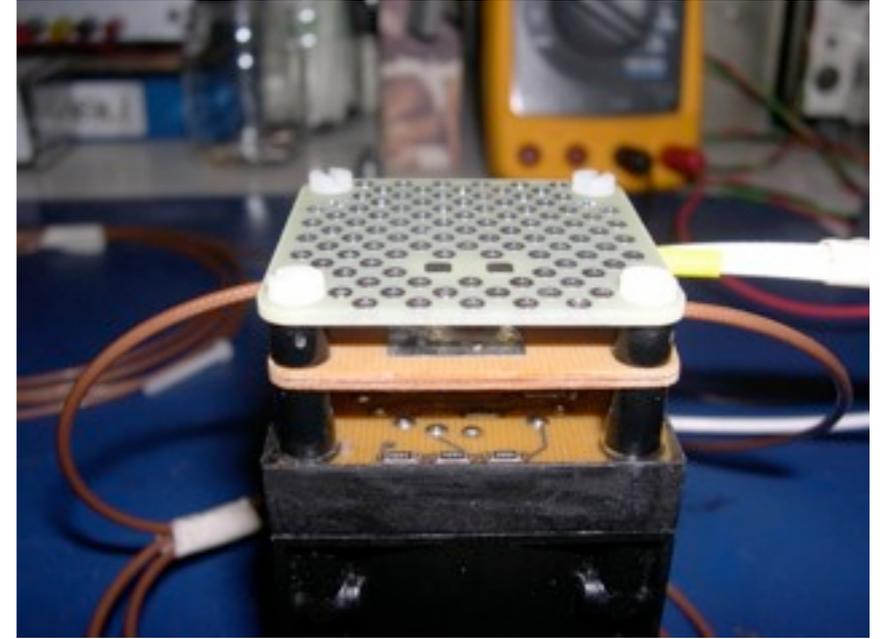
The PMT flying leads for the anode, the dynode and the PMT HV are soldered to the first card of the base.
