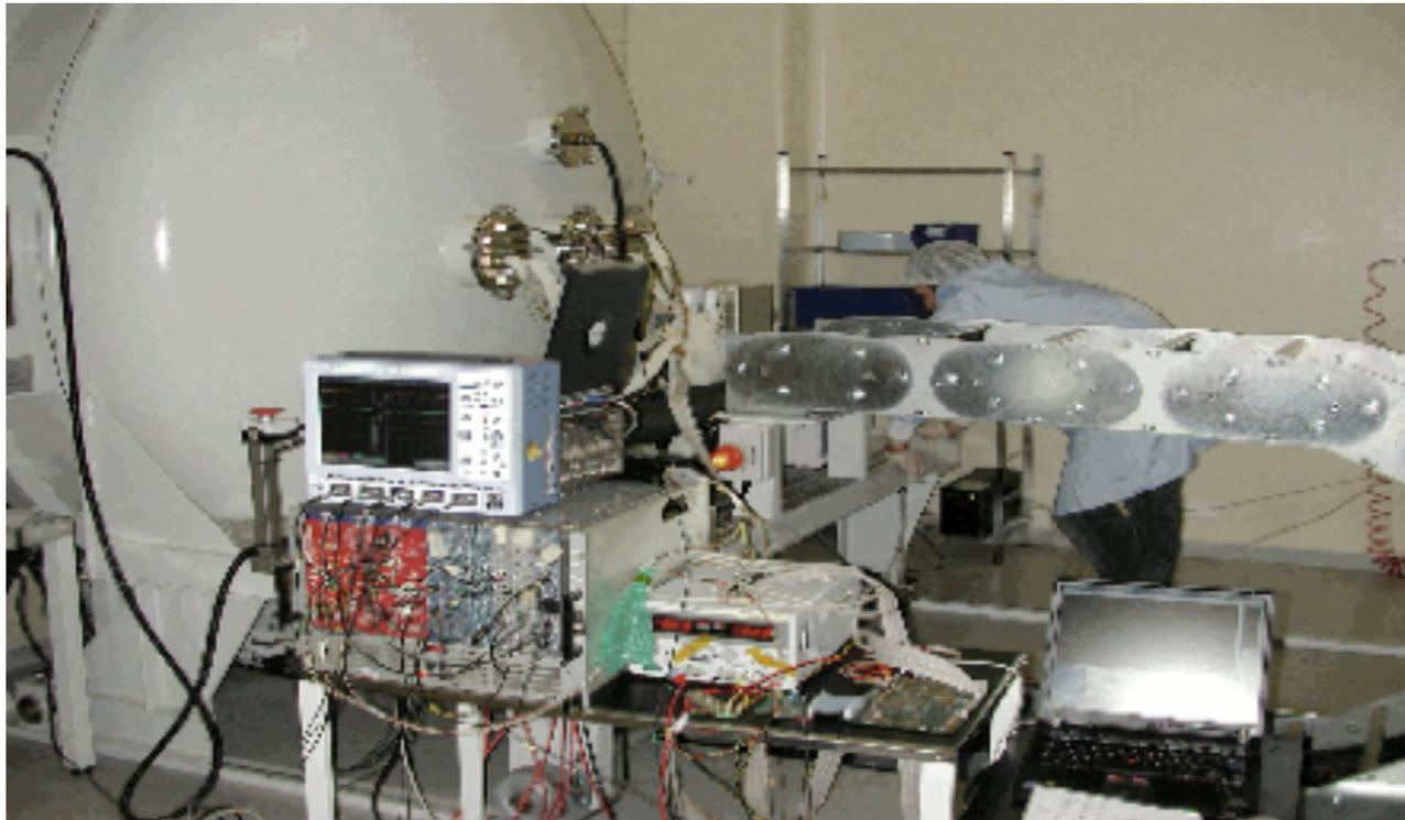
During the test, the pressure of the thermal vacuum chamber was about  $3 \times 10^{-5}$  mbar.
