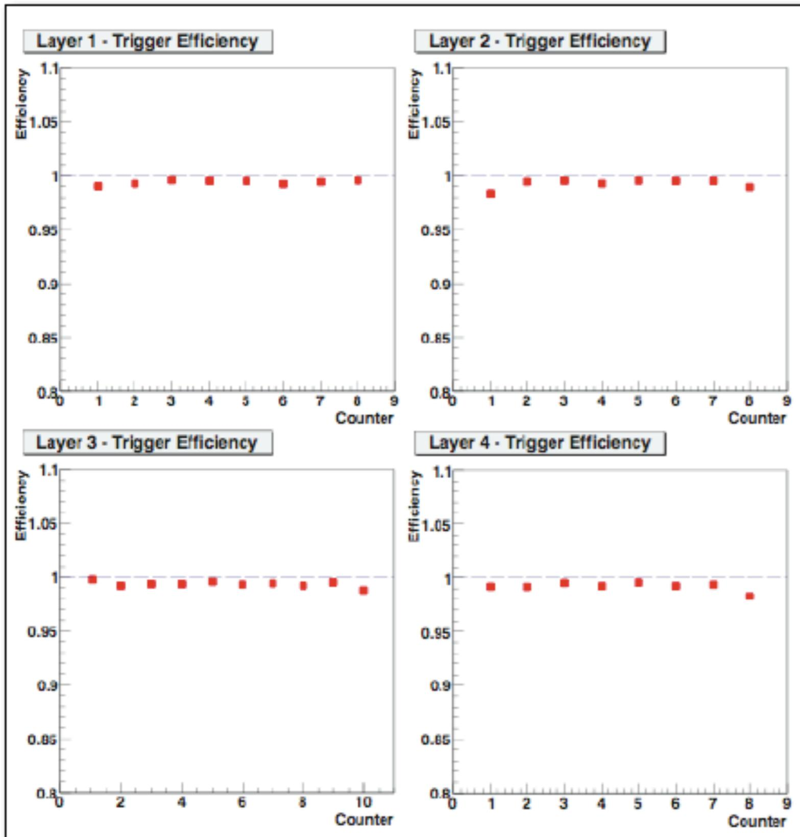
The efficiency of the counter is computed as the ratio between the number of events with any High Threshold in the counter and the total number of events with a particle hitting the counter.
