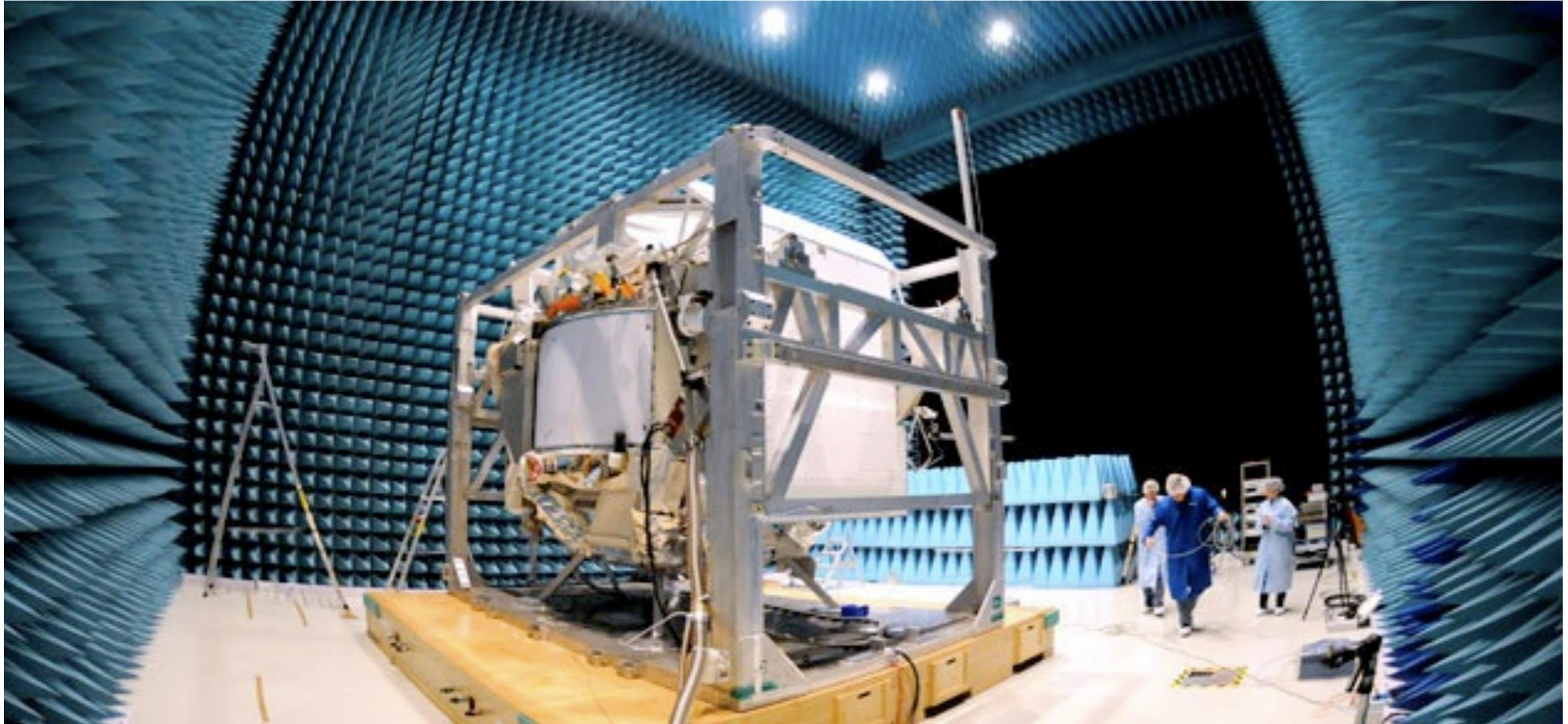
Electro Magnetic Interference test was needed to verify that TOF operations and performance were not adversely affected by the expected EMI environment of Shuttle and ISS and vice versa.
