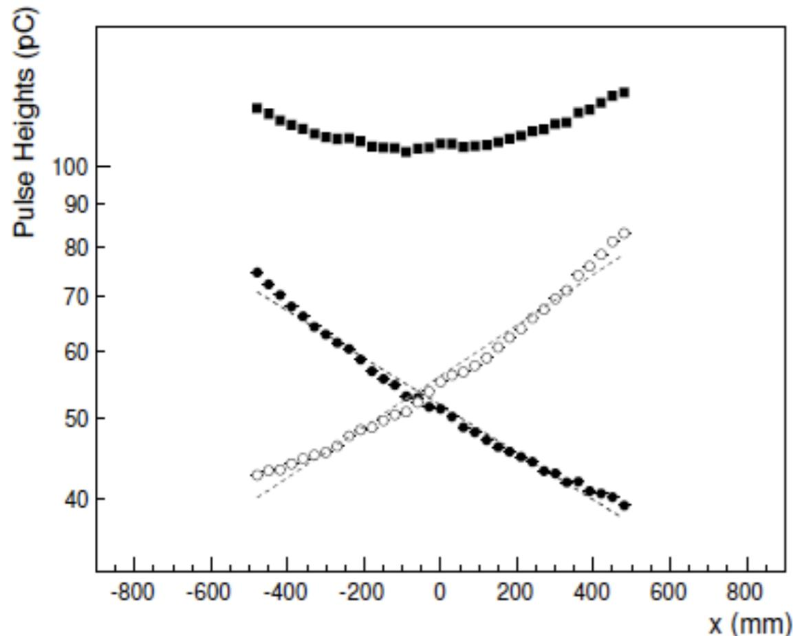
Pulse height for minimum ionizing particles as a function of the hit position along the counter; p side (white dots), n side (black dots) and sum of the two sides (black squares). The dashed lines are exponential fits to the data.
