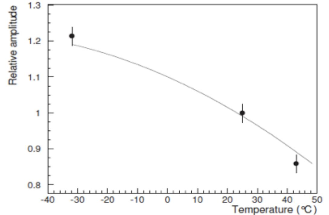
After vibration the mean anode amplitude in TOF layers 1, 2 and 4, relative to the amplitude before TVT, show a rather small decrease (about 10%) of the response, compatible with the scintillator accelerated aging due to the thermal stresses of the TVT test and the vibration.
