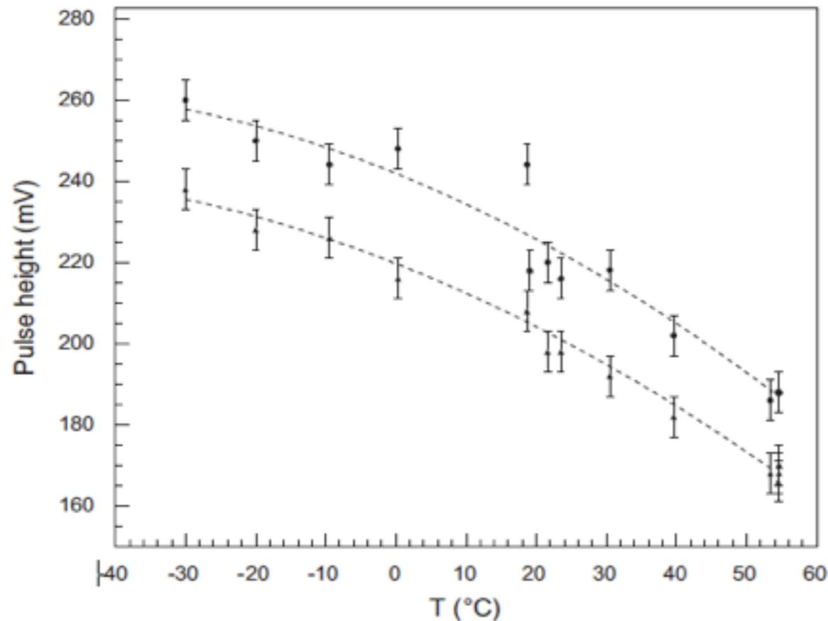
The variation of the pulse height as a function of temperature for two PMTs.
