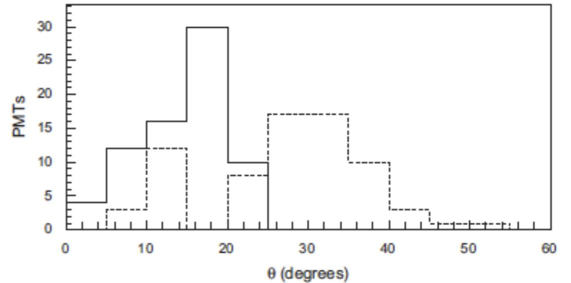
The resulting angle distribution with respect to the magnetic field for all PMTs. Full lines: layers 1 and 4. Dotted lines: layers 2 and 3.
