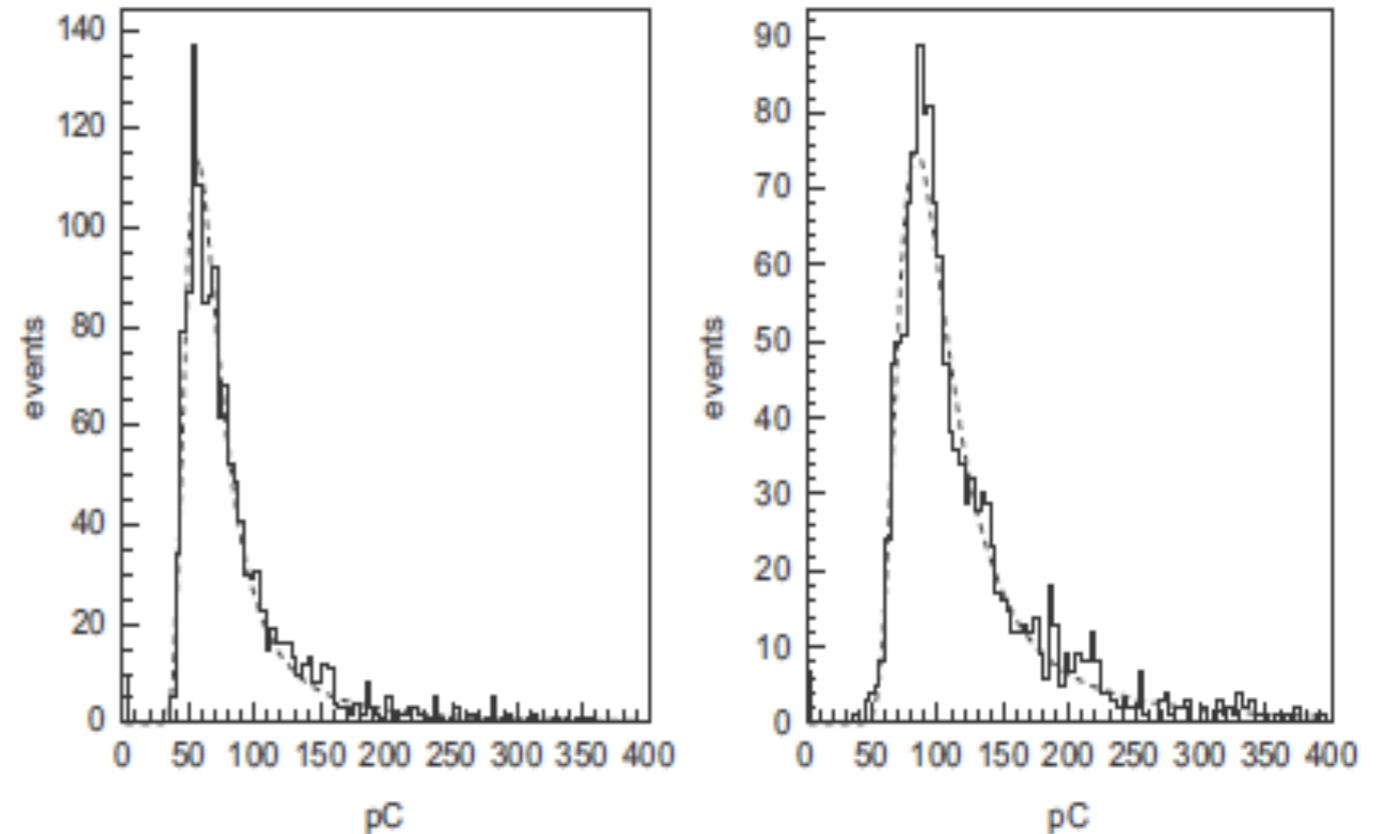
The anode pulse eight spectra of sides n and p of counter 402 for events selected in a 10 cm central section, fitted with a Landau shaped function.
