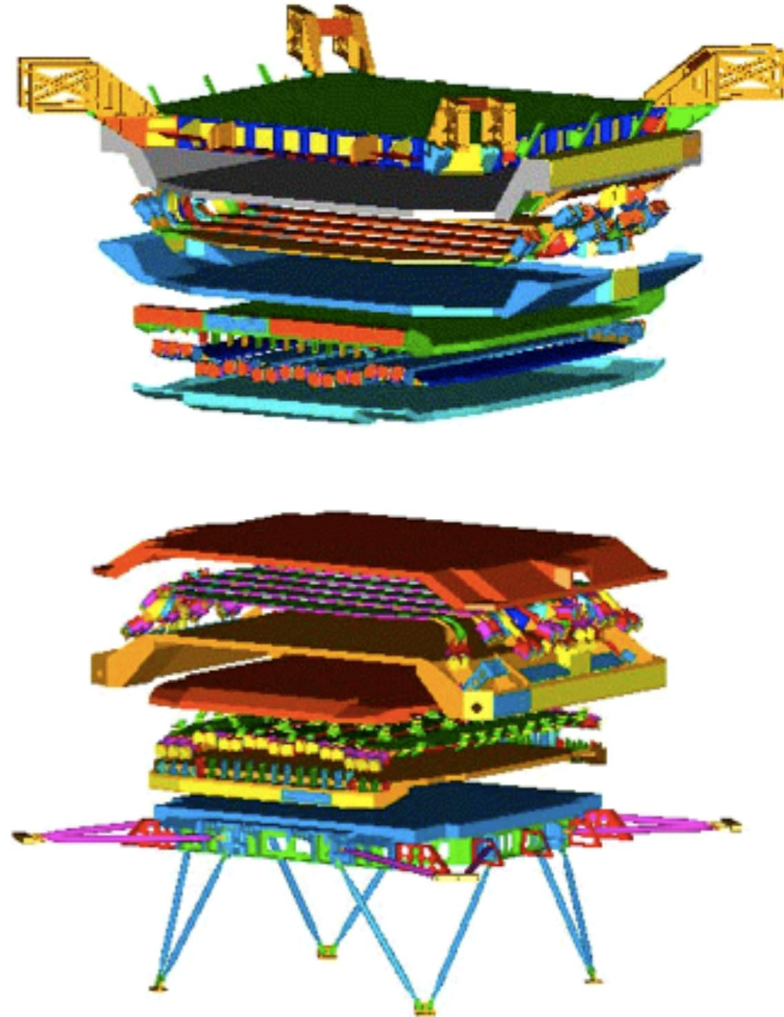
The exploded view of the mechanical structure of the upper and lower TOF
