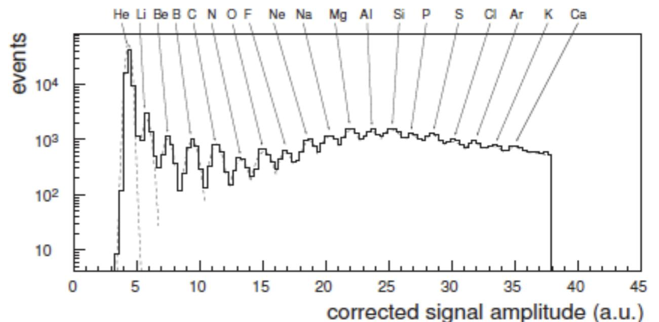
The amplitude spectra for different ions have then been corrected for the scintillator response.
