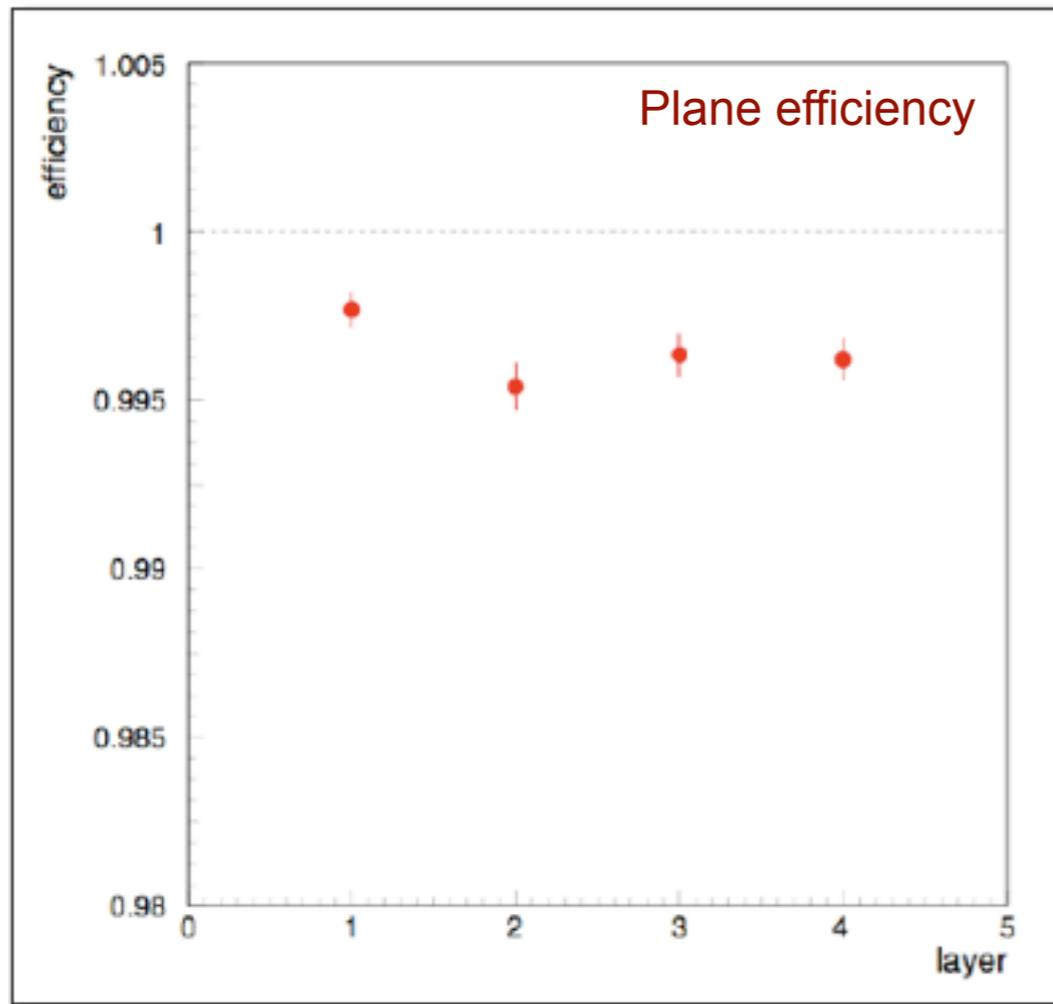
The efficiency of the plane is computed as the ratio between the number of events with any High Threshold in the plane and the total number of events with a particle hitting the plane.
