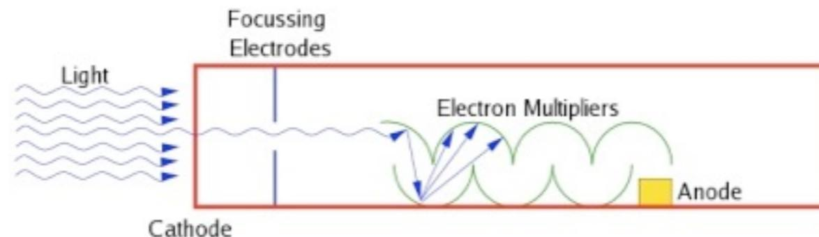
The electron multiplier consists of a number of dynodes. Each dynode is held at a more positive voltage than the previous one, so electrons are accelerated by the electric field and arrive with much greater energy. The geometry of the dynode chain is such that a cascade occurs with an ever-increasing number of electrons being produced at each stage.
