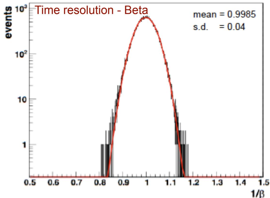
$\sigma$  ~ on beta 4% that corresponds to 180 ps single counter resolution (average flight path ~140 cm)
