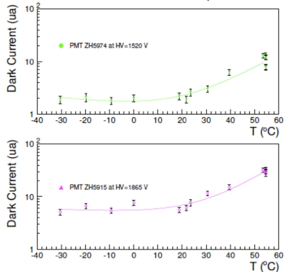
The variation of the dark current versus temperature for two PMTs.
