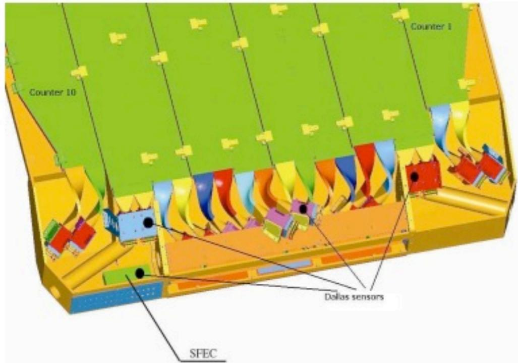
Temperature sensors are also located on SFET TDCs
